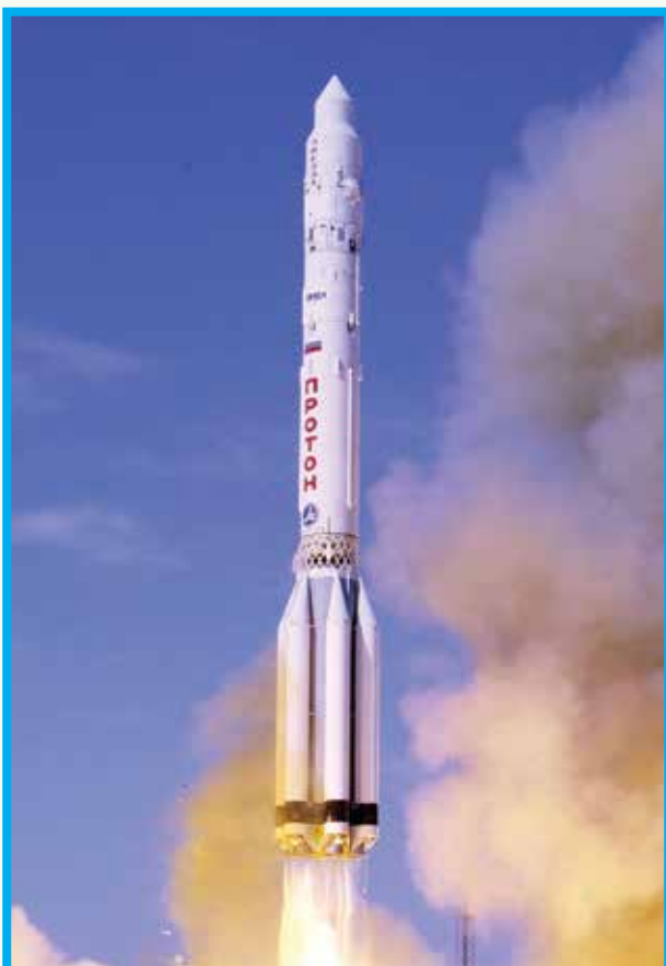
A Proton-K rocket being powered by the combustion of a fuel (hydrazine \text{N}_2\text{H}_4 ) and an oxidant (dinitrogen tetroxide \text{N}_2\text{O}_4 ).
