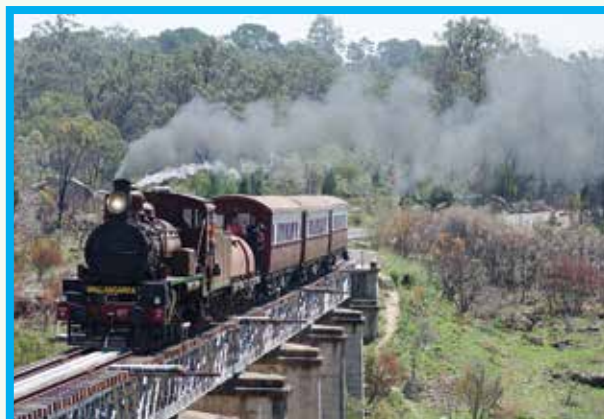
A steam train puffing sooty smoke - an indication of incomplete combustion.
