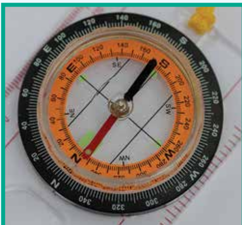
An orienteering compass. The red needle points to magnetic north.
