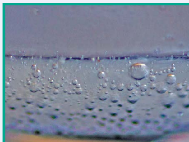
The reaction of vinegar and baking soda producing bubbles of carbon dioxide gas. The bubbles slow in activity as either the vinegar or baking soda are used up in the reaction.
