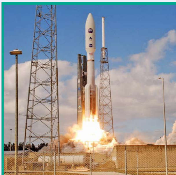
An Atlas V rocket using kerosene and liquid oxygen to power its first stage. The rocket uses liquid hydrogen and liquid oxygen to power the upper stage.
